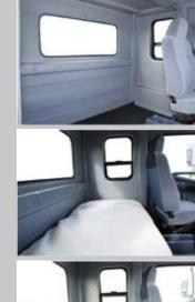
A fully-trimmed 30-inch cab extension is available with either a full-width bench seat, a 26-inch day bunk, or with the front seat configuration only. Side window vents add to driving comfort and a composite outer skin helps reduce corrosion. (Available on all models.)
