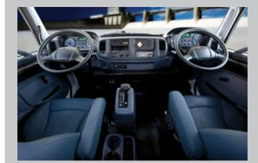
Driver controls are mounted on both sides of the cab specifically for dual steer applications where curbside diving visibility is important. The ignition switch is centrally-located; both seating positions are equally spacious; and with our original equipment parts, reliability and serviceability are built in. (Available on 258ALP, 268A, 338.)
