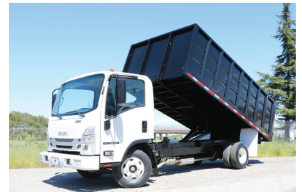
2025 Isuzu NRR 18ft Dump , V8 gas, automatic, ac, 7" digital display audio system with back up camera, power windows and locks, cruise control, heavy duty floor mat, solid steel container, 48" high steel sides, smooth steel bed, pull tarp system, swing out rear barn doors, 19,500 GVWR
